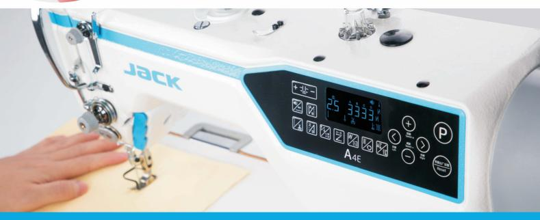
Computerized Lockstitch Machine With Electronic Control Stitch Length System
