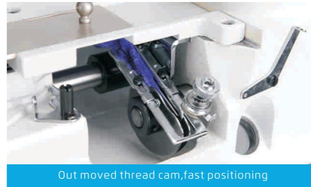
Out moved thread cam, fast positioning
