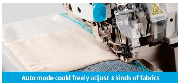
**Automatically adjust to fit with the thickness of fabric, change to corresponding sewing model**
