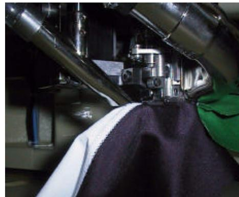
**MACHINE A BRAS DEPORTE TYPE "FLAT SEAMER", 4 AIGUILLES, 1 BOUCLEUR, AVEC SYSTEME DE PRE-RASAGE DES BORDS, COUPE-CHAINETTE A COMMANDE PNEUMATIQUE EN DEBUT ET FIN DE COUTURE**
