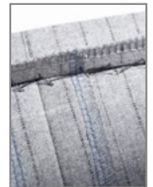
6. Hemming double blind stitch on skirts, unlined or half-lined jackets Class 352
