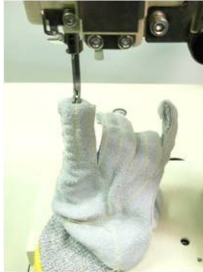
Suitable for sewing tubular part such as gloves' fingers
