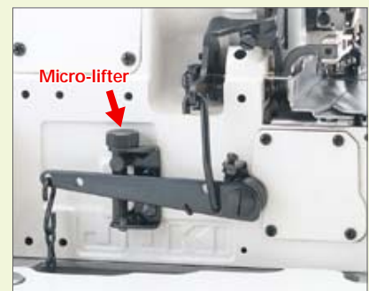
Bottom and top differential-feed micro adjustment mechanism
