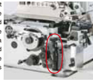
Differential-feed micro-adjustment mechanism
