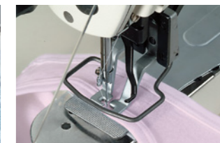
M type (Bartacking shoulder of running shirt)
