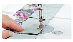
**Ever True Stitch Length** Ensures the truest stitch quality regardless of sewing speed. Also allows easy transition between different layers of fabric.
